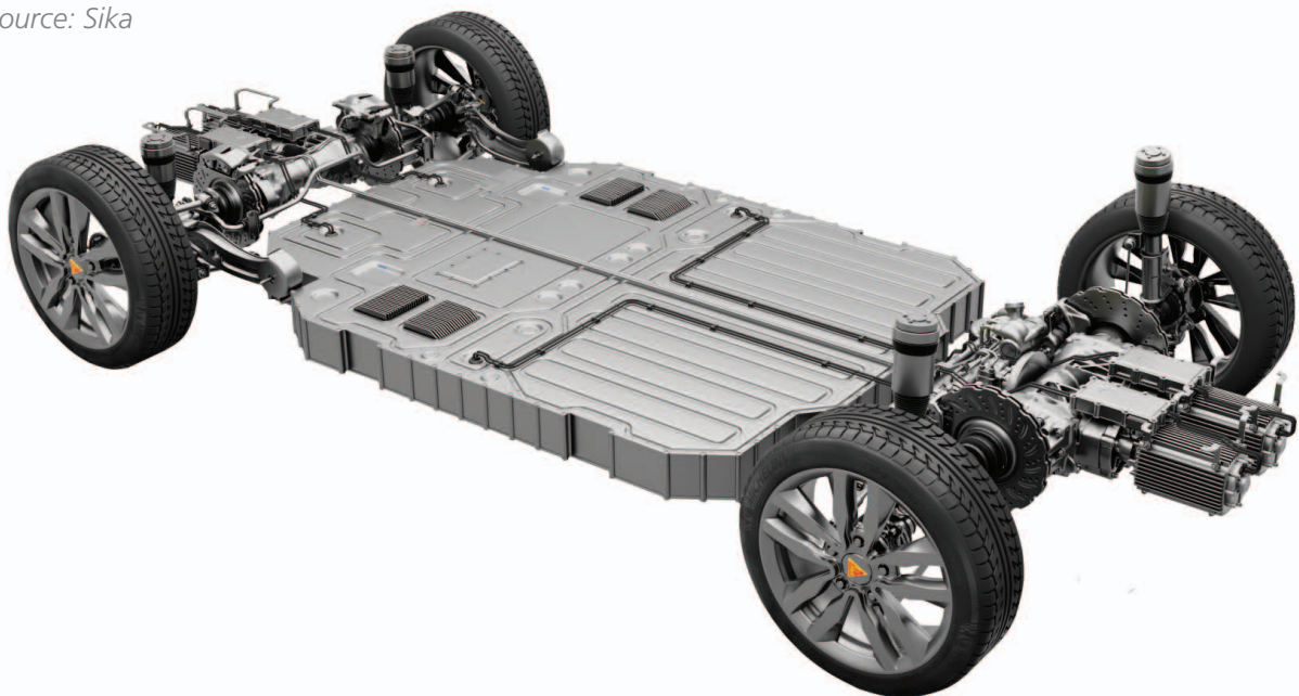
Figure 8: Light vehicle frame with battery pack installed
